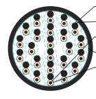
PVC Outer Sheath Tinned Copper Drain Wire Plain Annealed Copper Aluminium/polyester tape XLPE Insulation
